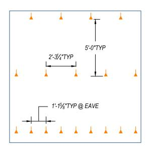
3 APEX D SNOW BRACKET LAYOUT DETAIL
